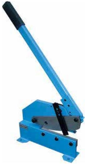
**Guillotine** For rough cutting out of shapes.
