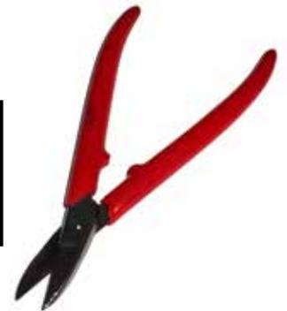
**Tip** - For cutting out rough shapes, use the guillotine or snips, but these distort the metal edges, so for neater, more precise cutting and intricate shapes you need to use a piercing saw.
