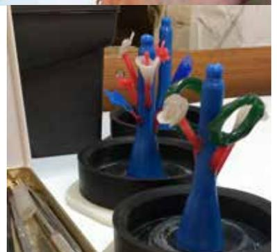
creating a new branch. This tree is set into a rubber base that is specially made to fit the casting canister.
