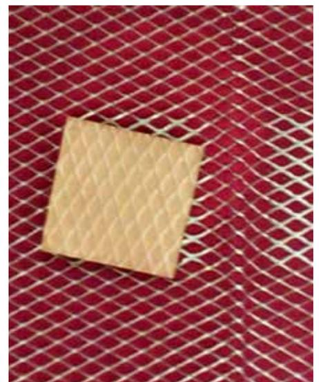
**Tip;** - Anneal (heat to soften) and then clean your metal before using hammers, punches or the rolling mill to ensure you get a crisp, clean imprint.
